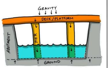
This is the simplest type of bridge with decking that \_\_\_\_\_s a gap supported by \_\_\_\_\_s on either side. Piers, which can help carry the load of the bridge, are sometimes used under the bridge in between abutments for added . When weight is exerted down on the bridge, the force/stress is spread and directed into the abutments and \_\_\_\_\_s.
