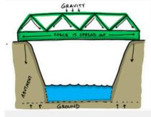
Like a simple beam bridge, the Truss Bridge uses decking across a span supported by abutments and sometimes piers. A truss bridge also has **triangle** sections across the deck that will carry different forces (tension and **compression**) ultimately to the ends (abutments). This spreads out the force across the deck, making the bridge stronger.
